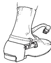
2. Fit the heel cup snugly to shoe and connect the Snap-Loc fastener together. Adjust elastic strap for comfortable fit. Tuck excess elastic strap behind itself.
