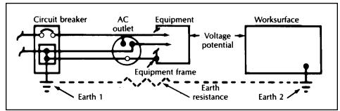
Figure 2. Separate ground systems present potential problems.
