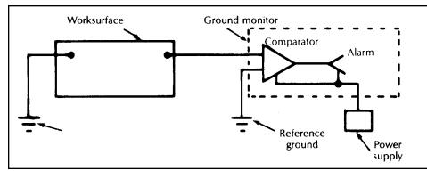
Figure 6. Block diagram of a ground-integrity monitor.
