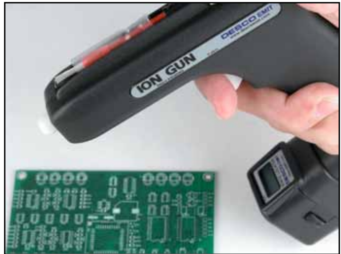
Figure 4. Using the EMIT Static Locator with the EMIT Ion Gun
