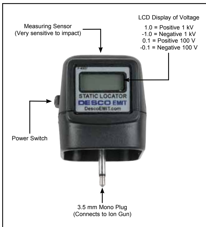
Figure 2. EMIT Static Locator Features and Components
