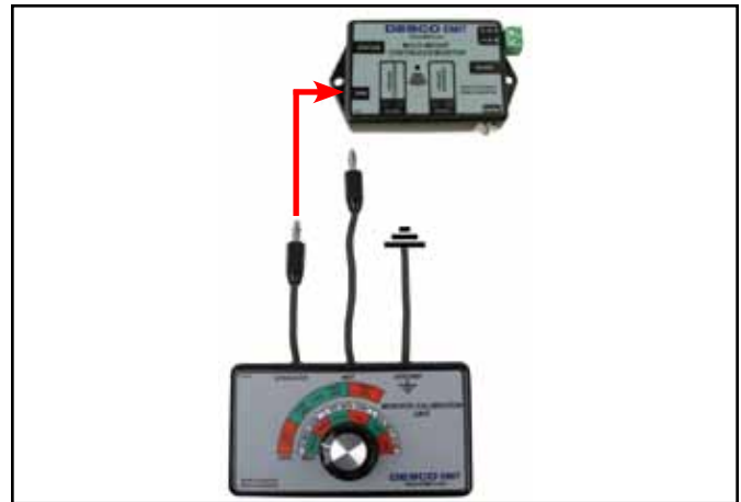
Figure 8. Connecting the OPERATOR test lead from the Monitor Calibration Unit to the Multi-Mount Continuous Monitor
