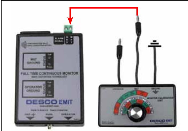
Figure 3. Connecting the MAT test lead from the Monitor Calibration Unit to the Full Time Continuous Monitor
