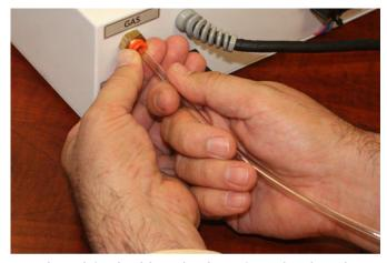
colored plastic ring with one hand (unlocking the hose) and using the other hand, pull the tubing from the fitting at the same time.
